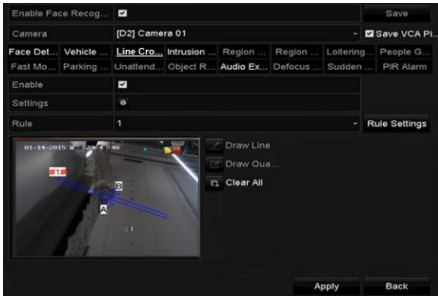
Figure 9. 2 Draw Line for Line Crossing Detection
