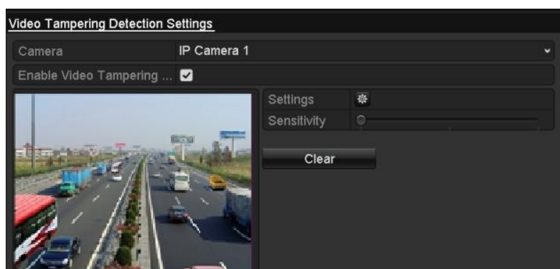
Figure 8. 11 Video Tampering Setup Interface
