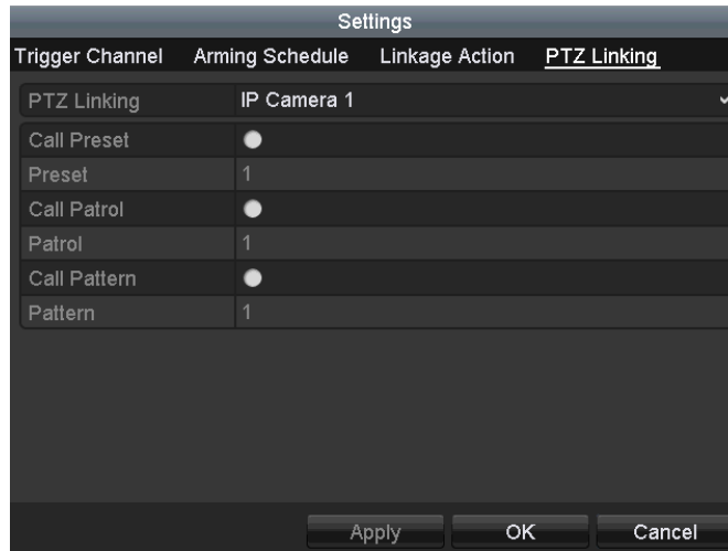
Figure 8. 7 Set PTZ Linking of Alarm Input
