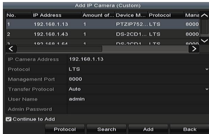
Figure 2. 18 Custom Adding IP Camera Interface
